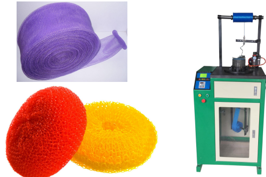
Plastic mesh scourer knitting machine
